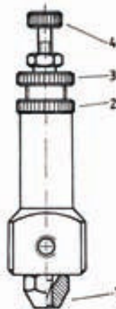
Type GV-E 1. Solid stream nozzle opens through self-pressure 2. Lock nut 3. Opening pressure regulation 4. Flow rate regulation
