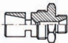
Type JM-K with head thread to be screwed into container's external wall, Dimensions on request
